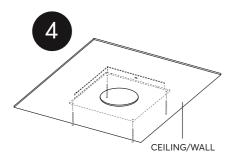
Mount the Speaker Back Box directly behind the plasterboard. Use min. 4x screws to secure the box behind the plasterboard.
